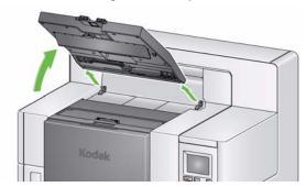
2. Remove the printer cover by placing your hand in the center back of the cover and pulling it straight up from the back edge.
