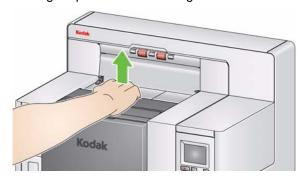
3. Install the Controlled Dual Stacking exit tray as shown below. Position the two latch handles to lock it in place.
