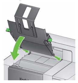
4. Install the extender insert for Stack #1 as shown
