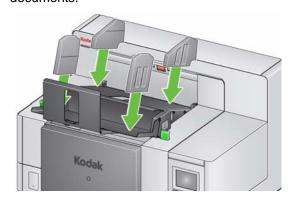
6. Using the thumbscrews on the bottom of Stack #2, adjust the exit tray to the length of the documents that will be output to Stack #2.
